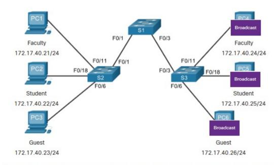
PC1 sends out a local Layer 2 broadcast. The switches forward the broadcast frame out all available ports.
