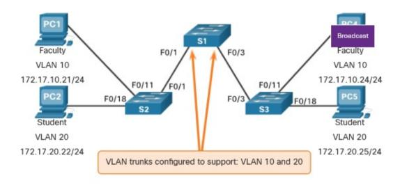
PC1 sends out a local Layer 2 broadcast. The switches forward the broadcast frame only out ports configured for VLAN10.
