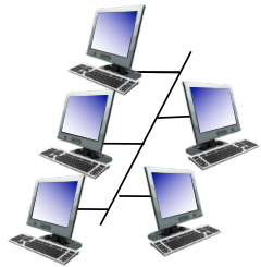
shared wire (e.g., cabled Ethernet)
