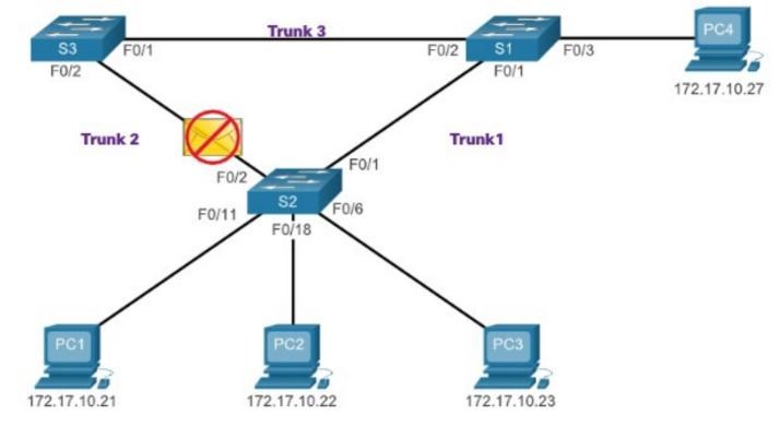
S2 drops the frame because it received it on a blocked port.
