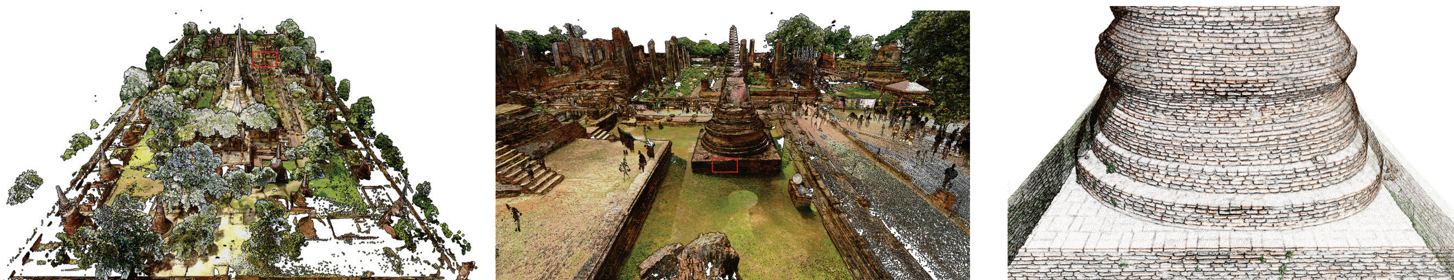
The site Wat Phra Si Sanphet, Ayutthaya (Thailand) resampled with our graph-based approach. Only 2.8% of the original 5 billions points (156 acquisitions) have been kept.
