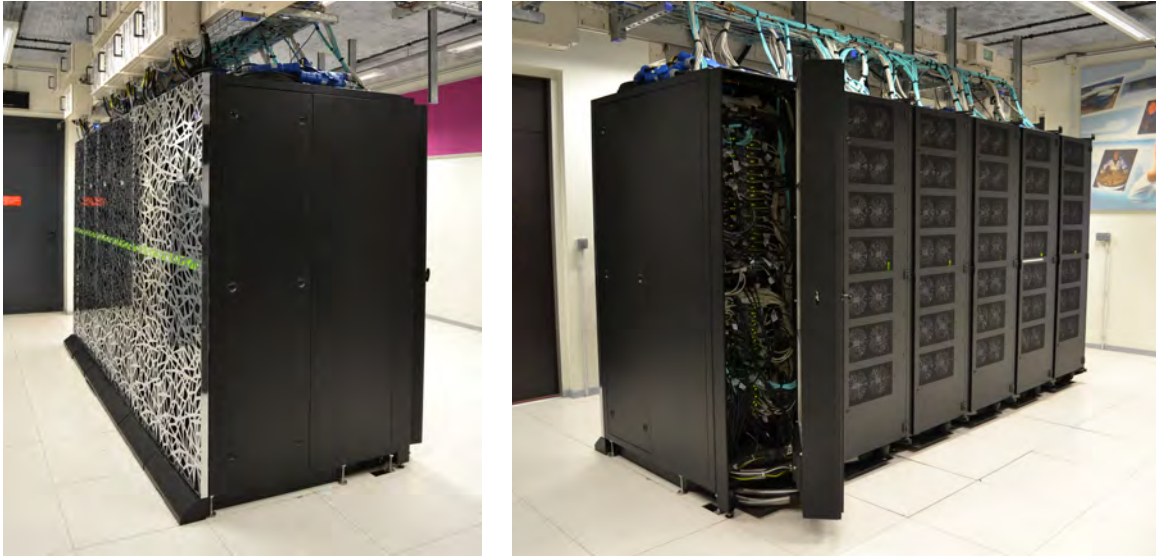
Figure 1.2: On left, a picture of the IFP Energies nouvelles supercomputer, called ENER440, at Lyon - Solaize, with details of its back (right picture) and its cooling doors equipped with cold water circuit 13 degrees.
