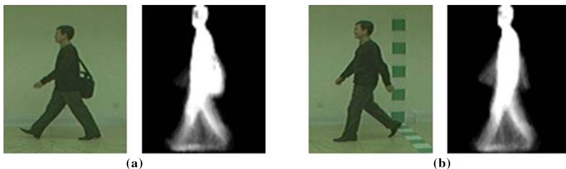
Fig. 6 A GEI image showing a person carrying single shoulder bag (a), carrying nothing (b)
