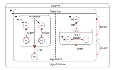
**Fig. 1.** A Typical SyncChart: This syncCharts specifies a detector of synchronized occurrences. Signal AB must be emitted when A and B have occurred, in any order, but "close enough" in time. "Close enough" means that there are at most two occurrences of T between the occurrences of A and B. Reset is a signal re-initializing signal. Finally, Inhib is a signal that enables "time suspension": when Inhib is present, possible occurrences of T are ignored.
