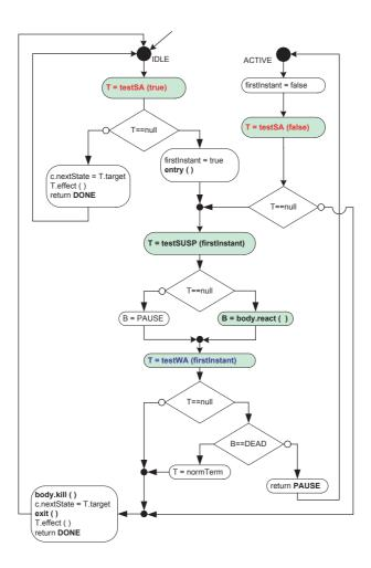
$\textbf{Fig. 8.} \ Reactive Cell \ Reaction: \ Reactive Cell: : \texttt{react()} \ method.$
