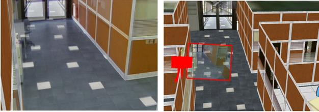
(b) Camera registration in (left) Augmented Reality mode with alpha blended video on 3D model and (right) Mixed Reality mode, the registered camera is represented by a red 3D object and the image plane in the sensor visual field of view.
