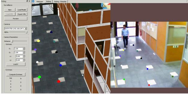
(a) Picking correspondences between (left) 3D model and (right) IP camera frame: matches points are represented with colored 3D spheres.
