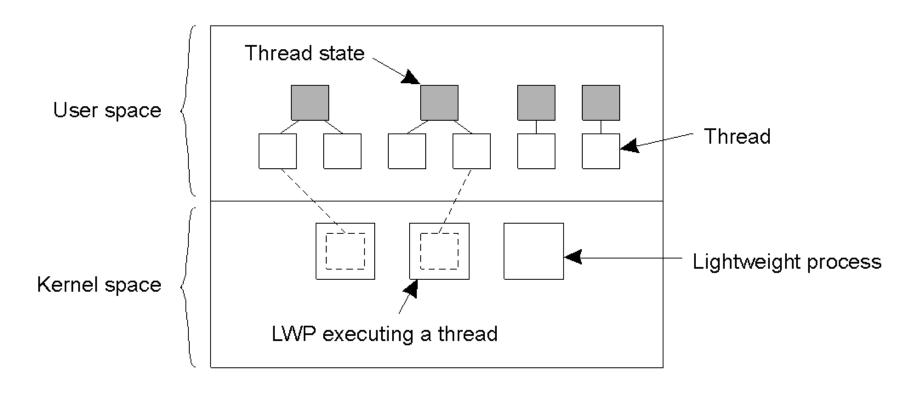
Combining kernel-level lightweight processes and user-level threads.
