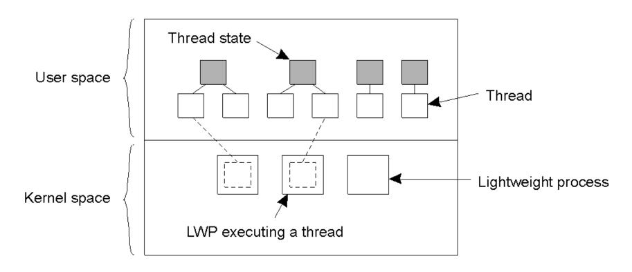
Combining kernel-level lightweight processes and user-level threads.
